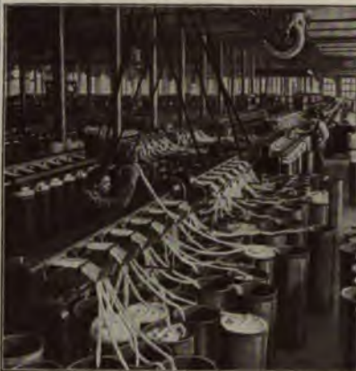
2. The cans containing the rolls which have been combed are placed in front of this machine. Five or six of the rolls are drawn out at one time, and afterward twisted together to make a cord which is wound upon big spools.
